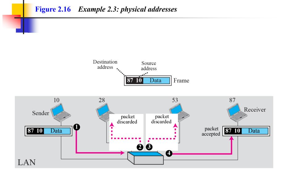
As we will see in Chapter 3, most local area networks use a 48bit (6-byte) physical address written as 12 hexadecimal digits; every byte (2 hexadecimal digits) is separated by a colon, as shown below:
