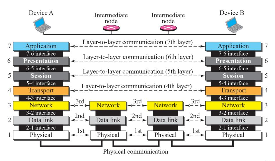
Figure 2.5 An exchange using the OSI model
