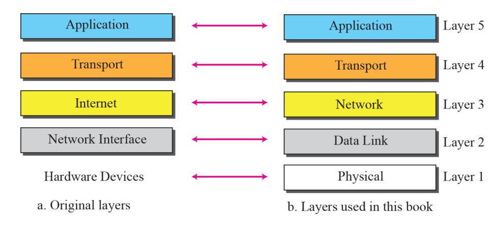
Figure 2.8 TCP/IP and OSI model
